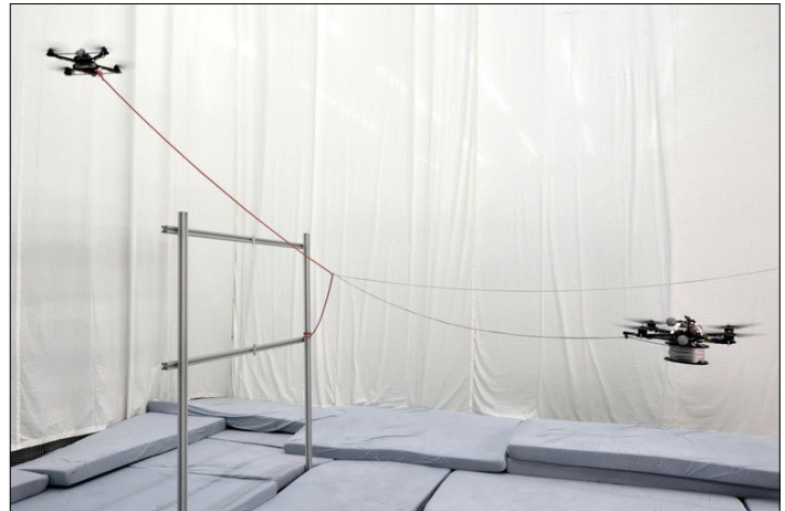
ETH Zurich investigating use of drones to build tensile structures
