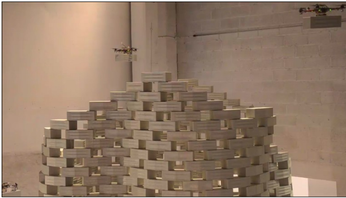
Drone assembling polystyrene brick structure
